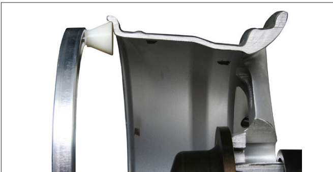
Figure 2 - Clip-On Weight Location
