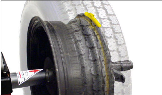
Figure 24 - Calibration Weight On Outboard Flange At Top-Dead-Center
