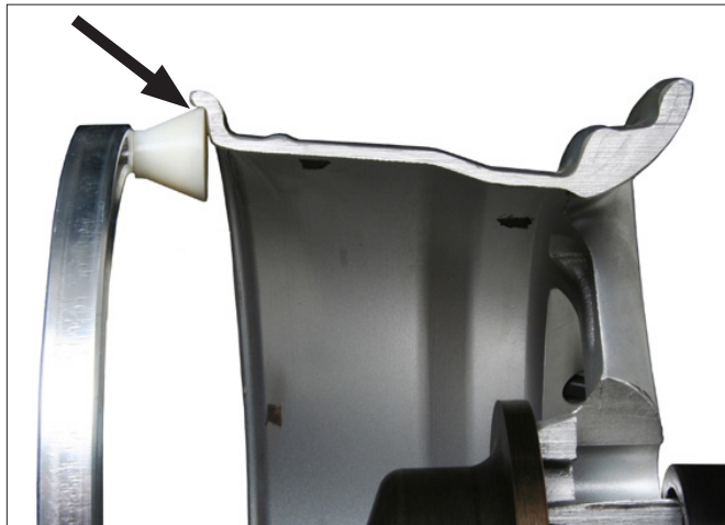
Figure 11 - Clip-on Weight Location Viewed on a Cut-Away Rim for Clarification.
