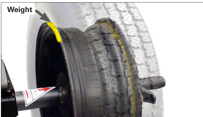
Figure 41 - Calibration Weight Moved (Directly Across) To Inside Flange
