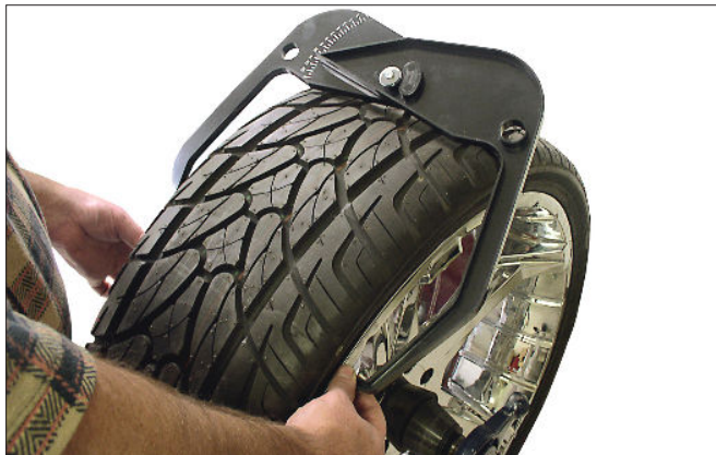
Figure 31 - Caliper Placement On Wheel
