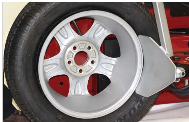
Figure 32 - Loosen Bottom Bead
