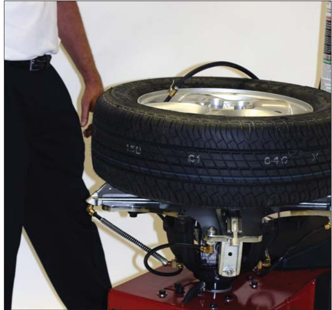
Figure 26 - Stand Back during Bead Seat
