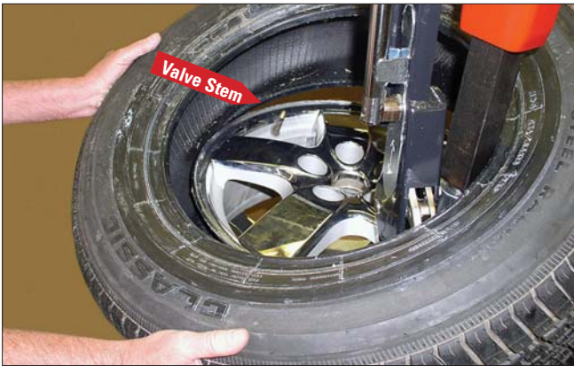
Figure 57 - Position Valve Stem in Front of Bead Lock
