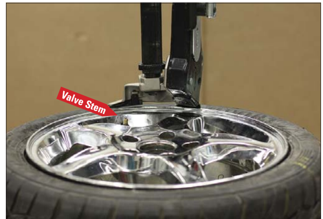
Figure 50 - Position Valve Stem Behind Leverless Demount Tool
