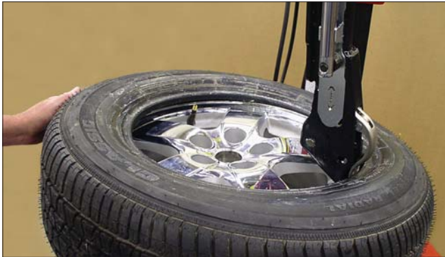
Figure 52 - Demount Upper Tire Bead
