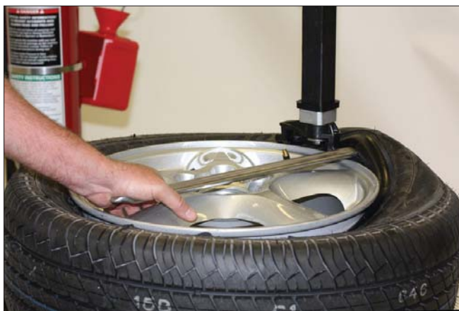
Figure 40 - Rotate Lifting Tool Down for Demount
