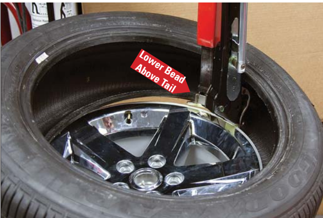
Figure 58 - Position Tire Against Bead Lifter Tool
