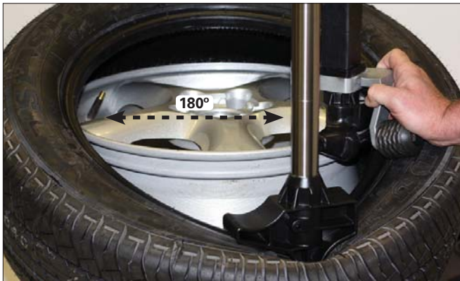
Figure 21 - Position Valve Stem 180° Ahead of Mount Tool
