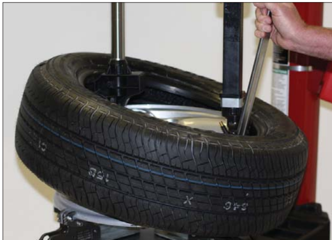
Figure 42 - Helper Holding the Lower Bead in Drop Center
