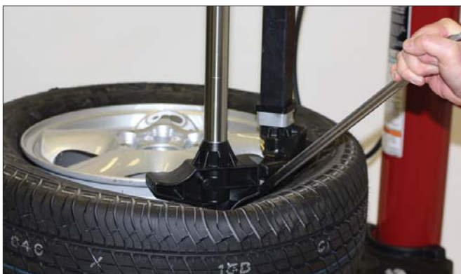
Figure 37 - Insert Bead Lifting Tool
