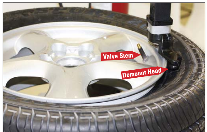
Figure 36 - Position Valve Stem Under Demount Tool
