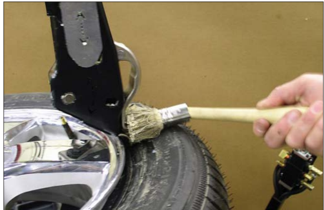
Figure 49 - Apply lubricant to Bead Lifter Tool Hook
