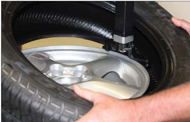
Figure 20 - Mounting Lower Bead
