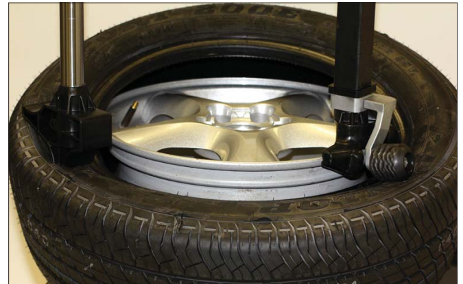
Figure 46 - Mounting Top Bead
