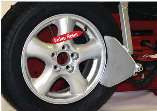
Figure 29 - Position Tire for Bead Loosening
