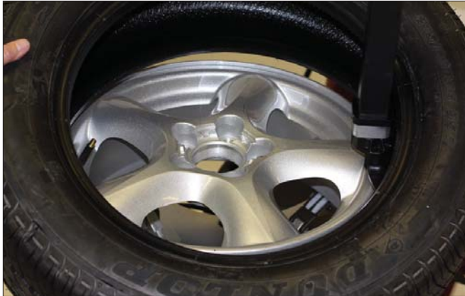
Figure 19 - Position Tire Against Mount/Demount Tool
