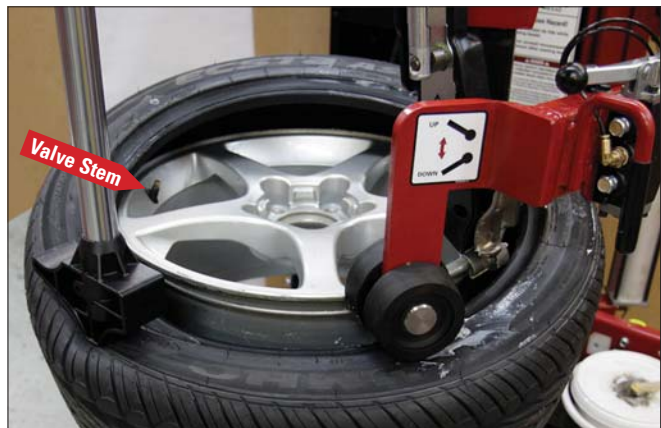
Figure 60 - Robo-Arm and Robo-Roller Pushing Tire Bead in to the Drop Center
