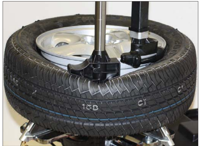
Figure 34 - Helper Foot Depressing Sidewall of Tire
