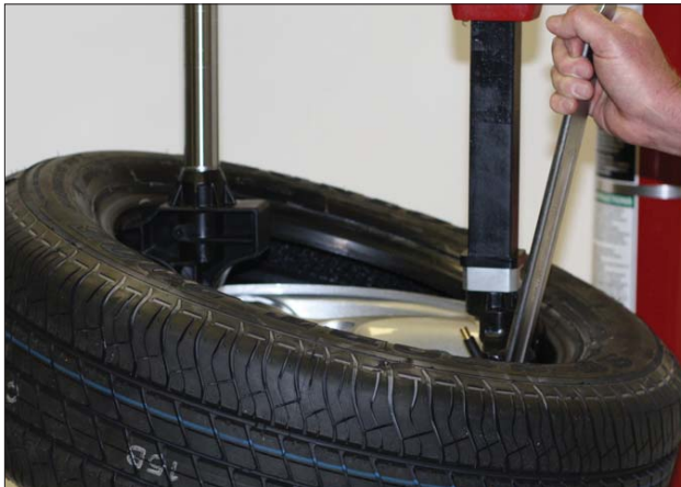
Figure 14 - Demounting Lower Bead
