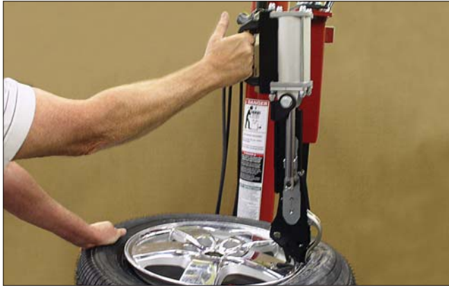
Figure 51 - Leverless Tool Hooked Under Tire Bead
