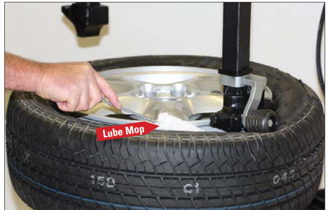
Figure 35 - Lubricate Upper Bead
