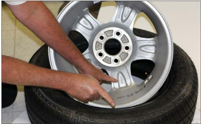
Figure 16 - Verify Size Match Between Tire and Wheel
