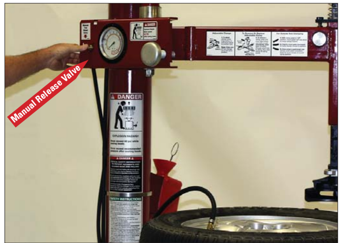
Figure 27 - Location of Manual Release Valve
