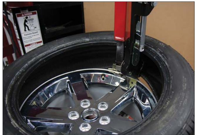
Figure 55 - Demount Lower Tire Bead
