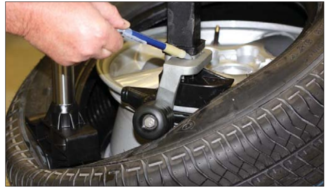
Figure 22 - Duckhead Roller Properly Mounted On Bracket
