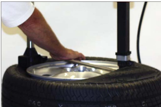
Figure 39 - Rotate Lifting Tool Down for Demount
