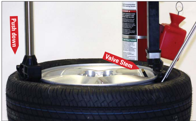
Figure 12 - Insert Bead Lifting Tool
