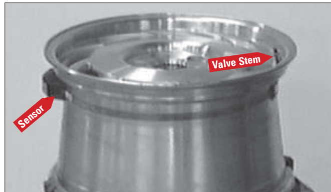
Figure 31 - Wheel with Low Pressure Sensor/Transmitter
