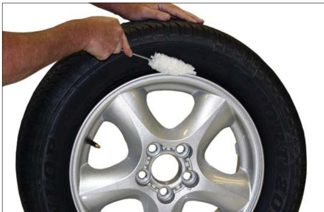
Figure 5 - Apply Rubber Lubricant to Tire Beads
