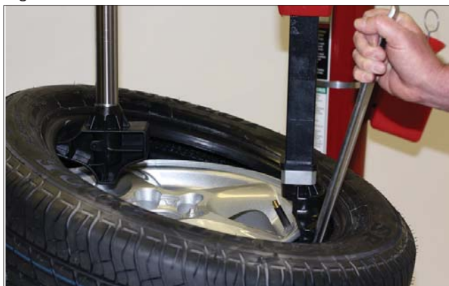
Figure 41 - Rotate Lifting Tool Down for Demount
