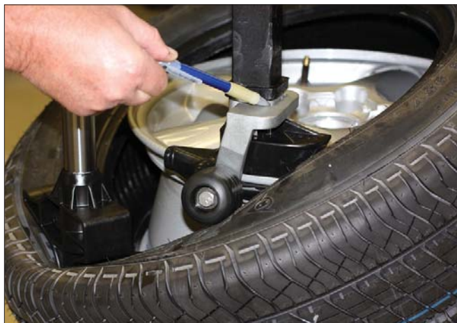
Figure 44 - Duckhead Roller Properly Mounted On Bracket
