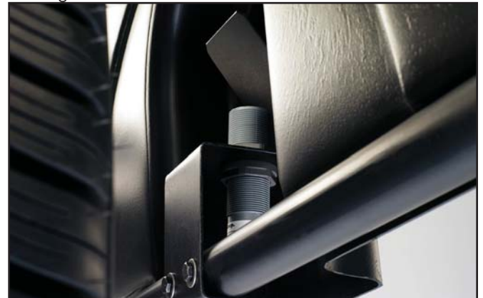
Figure 10 - Tire Width Sonar Located Inside Hood
