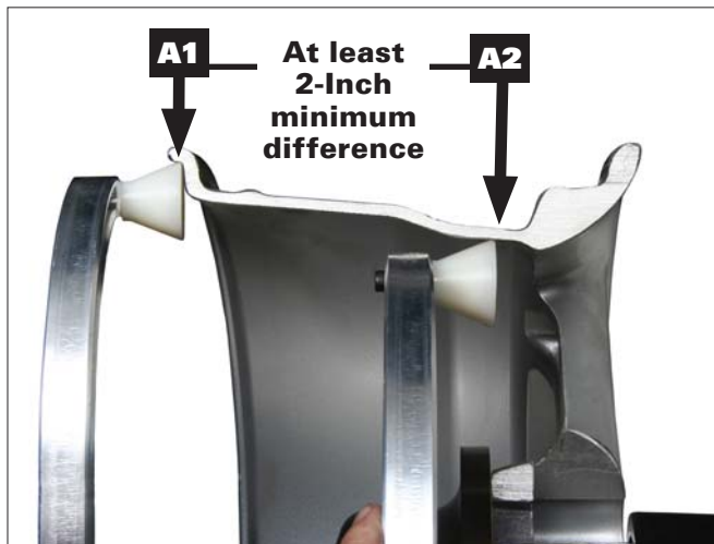
Figure 7B - T2-Tape (Hidden Tape-A-Weight®) Keep At Least 2-inches Between A1 and A2 Measurement
