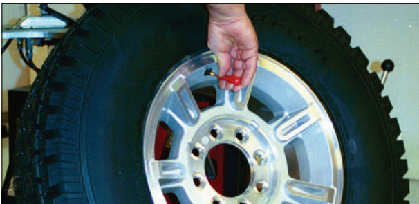
Figure 1 - Remove Valve Core to Deflate Tire
