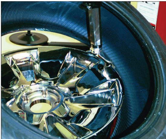
Figure 39 - Mount the Lower Bead
