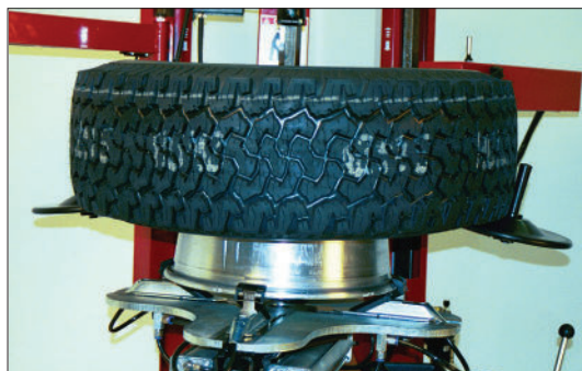
Figure 12 - Lift the Tire for Lower Bead Removal
