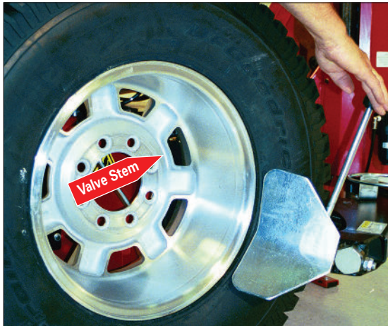
Figure 28 - Loosen Bottom Bead
