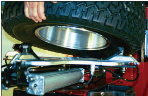
Figure 5 - Clamp Outside on Mag Wheels
