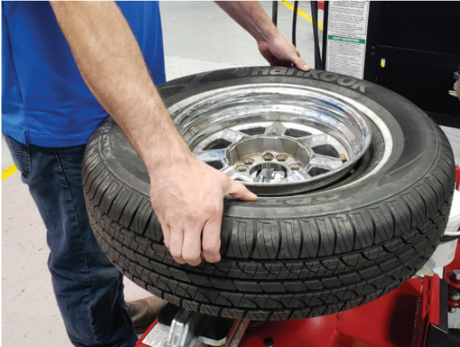
Figure 20 - Lift Tire Upwards for Bead Sealing
