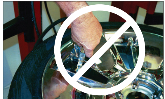
Figure 23 - Do Not Use a Hand-held Style Air Chuck
