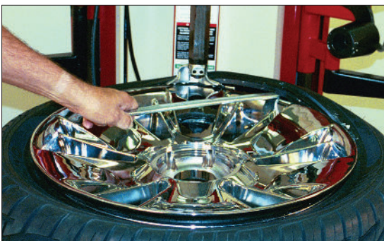
Figure 35 - Start Upper Bead Removal
