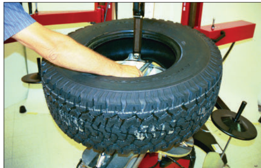
Figure 37 - Dismount the Lower Tire Bead from the Rim
