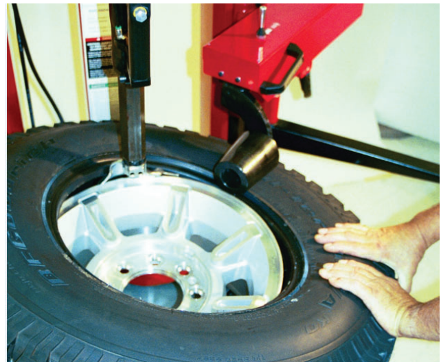
Figure 18 - Mounting Lower Bead
