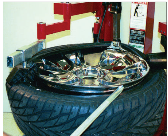
Figure 42 - Utilize the Lift Tool if Necessary
