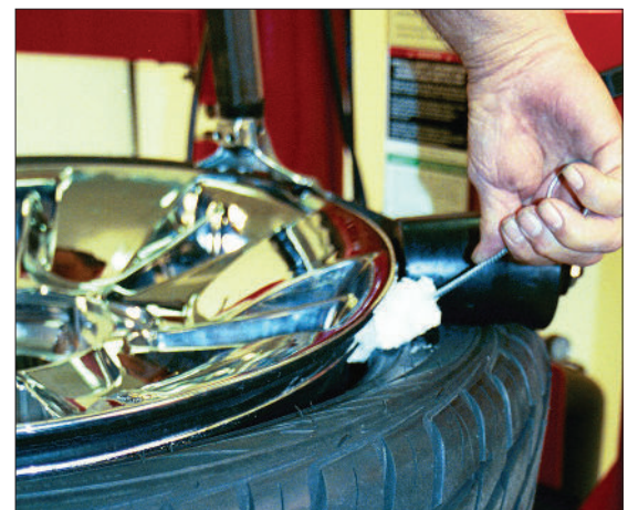
Figure 32 - Lubricate Upper Bead
