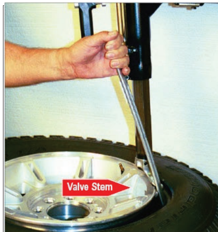
Figure 10 - Insert Bead Lifting Tool
