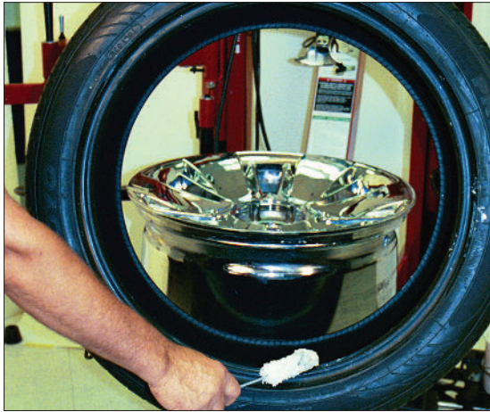
Figure 38 - Lubricate Tire Beads
