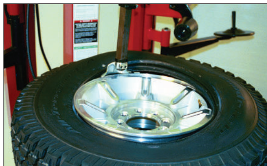
Figure 11 - Demount Upper Bead
