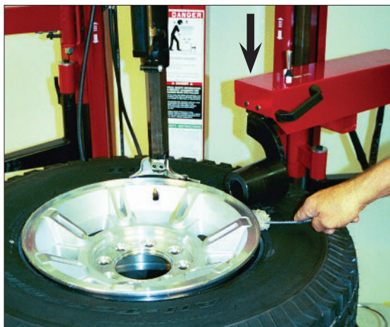
Figure 9 - Apply Rubber Lubricant to the Beads
