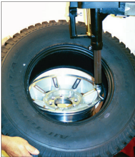
Figure 17 - Position Tire Against Duckhead Tool
