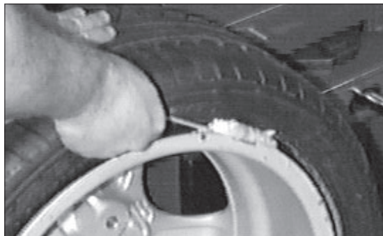
Figure 29 - Lubricate Bottom Bead
