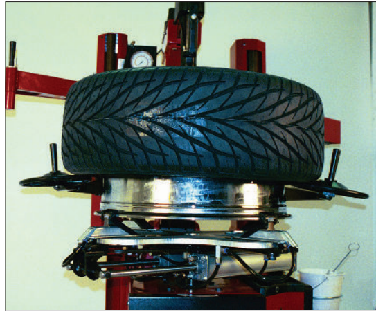
Figure 36 - Raise Lower Bead to Top of Drop Center of the Wheel
