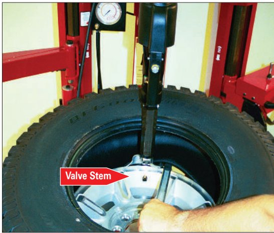
Figure 13 - Insert Bead Lifting Tool
