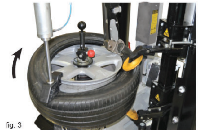
fig. 3 Press the pedal 2 to rotate the wheel clockwise, contemporarily press the tire manually from "5 o'clock" position to force the upper bead at drop-centre position. Keep it pressed while rotating up to "8 o'clock" position to complete the upper bead mounting (fig. 2).
