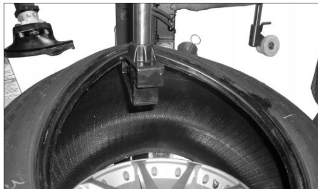
Figure 13 - Lift the Tire for Lower Bead Removal
