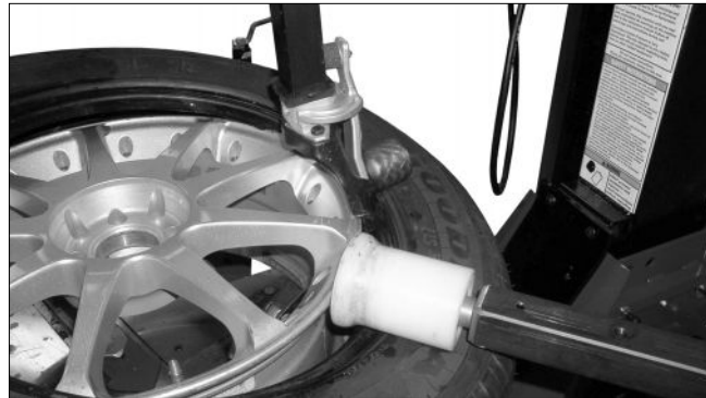
Figure 21A - Use Power Roller To Hold Tire In Rim Drop Center
