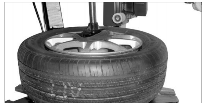
Figure 7 - Robo Arm Aids Clamping
