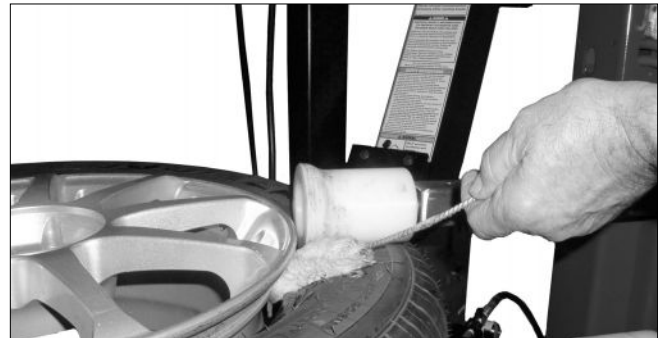
Figure 10 - Apply Rubber Lubricant to the Beads
