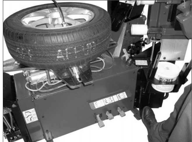
Figure 24 - Stand Back during Bead Seat
