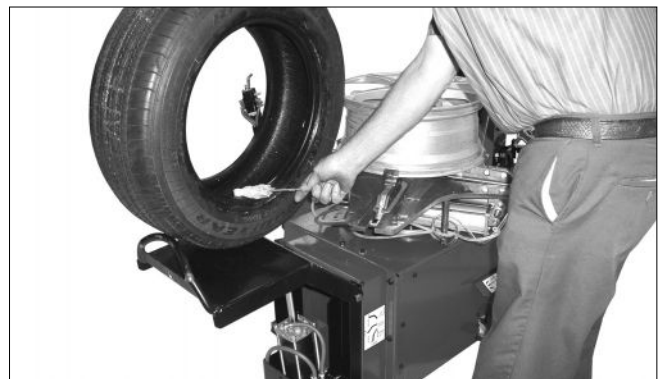
Figure 17 - Lubricate Tire Beads Liberally
