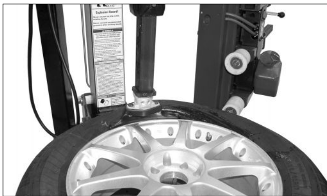
Figure 12 - Demount Upper Bead
