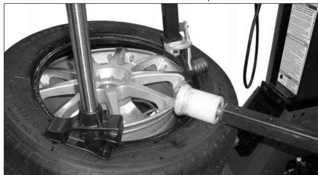
Fig 21B - Use RoboArm To Hold Tire In Rim Drop Center
