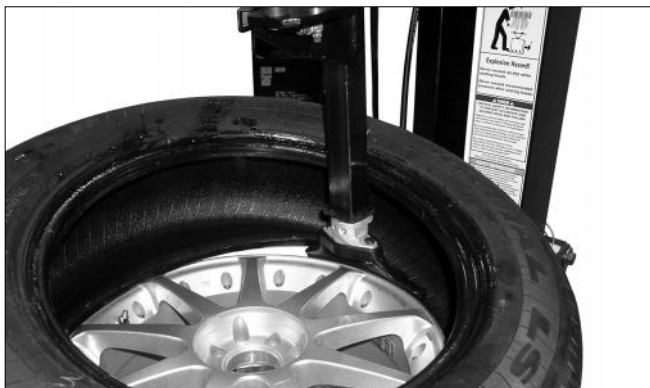
Figure 19 - Mounting Lower Bead
