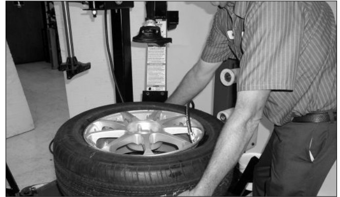
Figure 23 - Lift Tire Upwards for Bead Sealing
