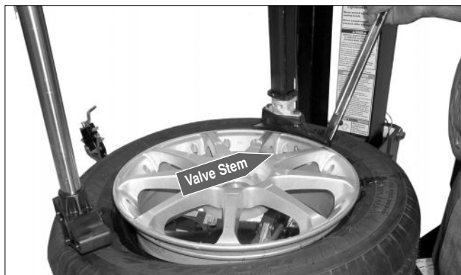
Figure 11 - Insert Bead Lifting Tool
