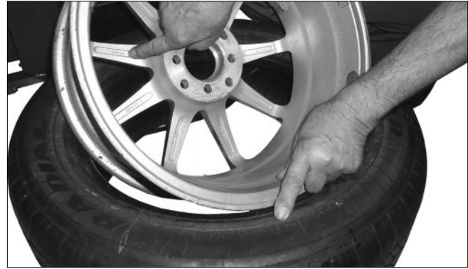
Figure 15 - Verify Size Match Between Tire and Wheel
