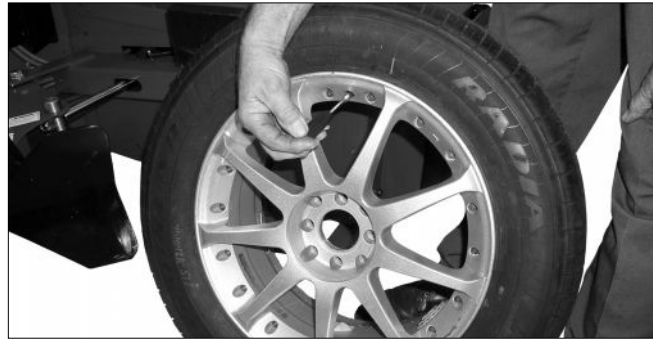
Figure 1 - Remove Valve Core to Deflate Tire
