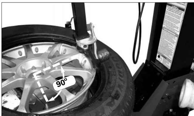
Figure 20 - Position Valve Stem 90° Ahead of Duckhead
