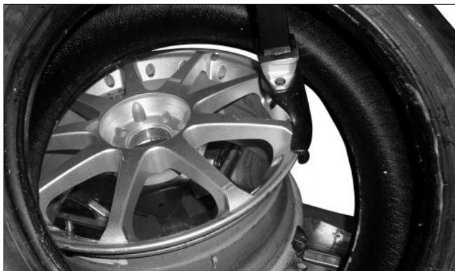
Figure 18 - Position Tire Against Duckhead®
