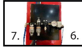
6. Air release locking system with regulator, filter oiler
