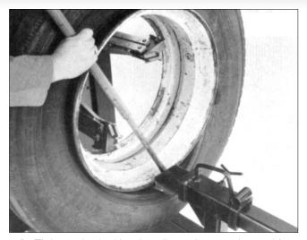
**3.** Tighten the locking handle and move the tool into position near the edge of the rim, as shown above.
