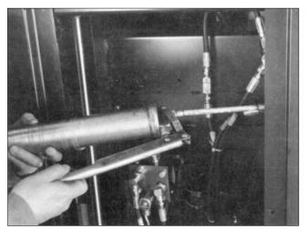
**2.** Remove the side panels and lubricate the four posts that guide the carriage up and down. Also, with a grease gun, lubricate the bushing sprocket tube. Lubricate these parts at lease once every month.
