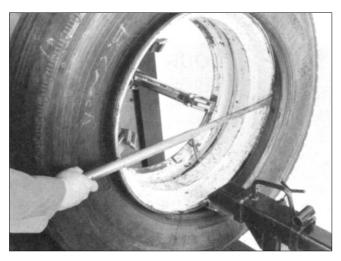
**5.** Pry the bead out over the rim. **Note:** You may have to assist the bead opposite the tool into the drop center. Use one of the tire tools to pry the top bead into the drop center.
