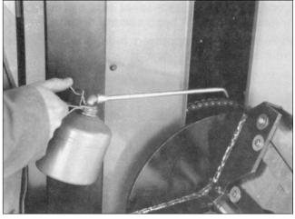
**3.** Using a grease gun and chassis grease, lubricate the disk shaft on the bead roller tube once every month.
