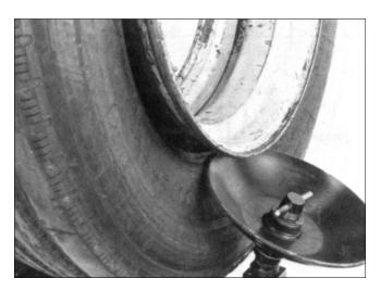
**3.** Rotate the tire. While the tire is rotating, slowly advance the bead loosening disc to contact the tire bead. Adjust the chuck up or down so the disc is close to the rim.
