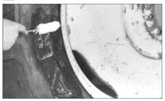
**Note:** Apply a liberal amount of lube to the tire sidewall. This will regain some of the original flexibility of the rubber, thus reducing possible damage to the sidewall.
