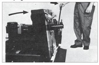
**1.** Raise working table: Raise working table to almost vertical position by pulling back on the control handle. Open clamps by twisting the control handle counterclockwise.
