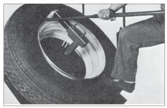
**2.** <u>Lift Top Bead:</u> Insert bead lifter under top bead to left of mount/demount tool and lift bead over lower blade of the tool head. Note: Make sure the top bead at the 6 o'clock position is in drop center.
