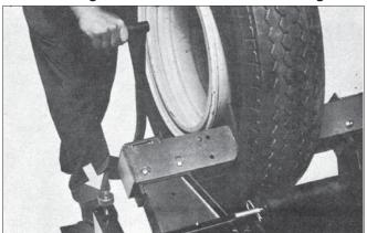
**2.** Adjust shoes and loosen beads: using handle, adjust bead loosener shoes on tire sidewalls 1/4-inch from rim contour. Depress left side of foot pedal to loosen beads. Depress right side to retract shoes. Note: for handling several wheels of the same size, an adjustable stop is provided for convenience. (See arrow.)
