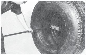
**6.** <u>Insert Bead Lifter:</u> With bottom bead in drop center and tire resting on the floor, rotate tool to 9 o'clock position and insert bead lifter under bottom bead just below the tool head.
