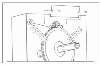
**6.** Lubricate Ring Gear: To gain access to the pinion and ring gear, remove the COATS name plate located on the working table. With a small brush or grease gun, apply AGMA #1 or #2 grease liberally on the ring gear teeth.
