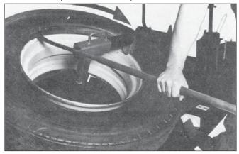
**3.** <u>Demount Top Bead:</u> Holding the bead lifter down as shown, depress the front side of either foot pedal thus rotating the tool head clockwise and demounting the top bead. Make sure mount/demount tool does not rotate into bead lifter during the operation.
