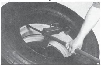
**4.** <u>Demount Bottom Bead:</u> Return mount/demount tool to the 12 o'clock position and insert bead lifter under bottom bead to the left of head. Again, make sure the opposite side of the bottom bead goes into drop center. Lift bottom bead over tool blade. Hold the bead lifter mount/demount tool clockwise and demounting bead. Make sure tool does not rotate into bead lifter during the operation.
