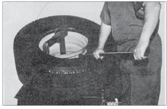
**3.** Mount Top Bead: Use bead lifter to hold top bead into drop center while tool rotates.
