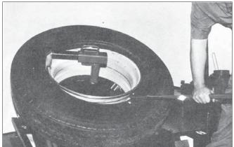
**6.** Mount Top Bead: With tool head at approximately the 7 o'clock position, push top bead over tool head and hold bead into rim drop center with the bead lifter as shown. Depress front of right foot pedal, thus rotating
