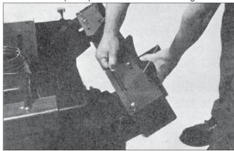
**1.** Adjust Bead Loosener Shoes: For tire width of 10" and over, one or both bead loosening shoes should be adjusted.
