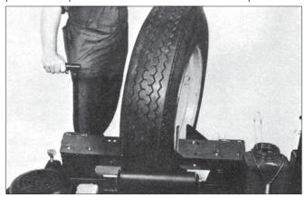
Angle Tire: (not recommended for aluminum rims) The shoe with the rim stop may itself be used as a rim stop. Angle the wheel so that this shoe contracts the rim and the opposite shoe contacts the unloosened bead.
