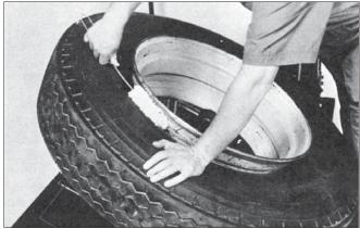
**5.** <u>Lubricate both beads thoroughly:</u> Both beads and the rim flange should be thoroughly lubricated with an approved tire lubricant before attempting to demount the tire. It may be easier to lubricate the bottom bead while the tire is in the bead loosener.
