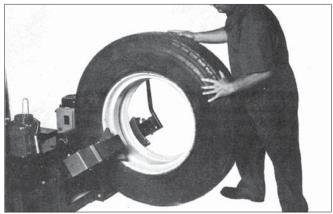
Roll Wheel: Retract shoes completely. Roll wheel forward firmly against the rollers and rotate it to a new position. Reposition and loosen bead as in step 2 above.
