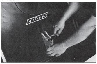
**2.** <u>Clamp Adjustment:</u> Adjust all three clamps to the proper wheel diameter range. The front hole position is for 19.5" to 24.5". The rear hole position is for 16" to 19.5".
