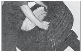
**3.** <u>Clamping:</u> Due to the stiff sidewall, it may be necessary to push down on the rim at the top as the clamps are being closed, to engage the rim. Lowering the table slightly will let the wheel's weight help in clamping.
