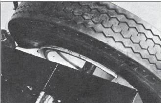
**4.** <u>Clamp Rim:</u> With the left hand on the top front of the rim, push the rim toward the upper two clamps. Then close the clamping jaws by twisting the control handle clockwise. Observe the clamping action to make sure all three clamps are properly engaged. Lower working table to desired angle by pushing forward on control handle.
