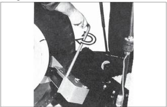
**3.** Actuate bead loosener so that the bead loosener shoe pushes bead in. As the kicker shoe passes the ring, pull handle to bring the kicker shoe up to the bead. Continue to full stroke of bead loosener.
