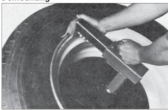
**1.** <u>Install Mount/demount Tool:</u> Insert mount/demount tool in square drive socket and position tool head on the rim flange. Rotate the tool head to approximately a 12 o'clock position by depressing either foot pedal.
