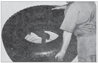
**1.** <u>Mount Bottom Bead:</u> With the table at a comfortable angle, mount the bottom bead in the usual manner. It may be necessary to lift the bottom bead into drop center as the mount/demount tool rotates.
