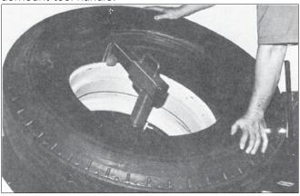
**5.** Mount Bottom Bead: Depress front of either foot pedal, thus rotating the tool clockwise. Hold down on the tire until the tool begins to mount the bottom bead. Make sure the bead goes into drop center behind the tool head.
