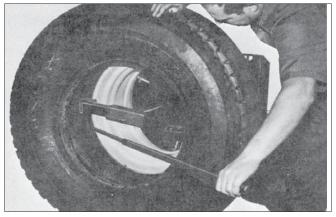
**7.** <u>Demount Bottom Bead:</u> Lift bead over mount/demount head. Rotate tool clockwise to demount bottom bead.
