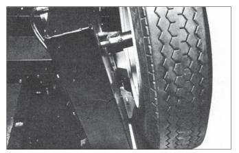
**3.** <u>Position Wheel:</u> Roll wheel onto the safety skirt as close to the working top as possible. Position rim flange into the lower clamp.
