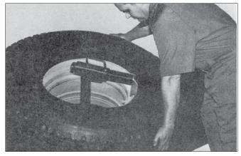
**2.** <u>Position Top Bead:</u> Manipulate and position the tire so that the bottom bead slips down toward its bead seat and the top bead rests evenly around the upper rim flange.
