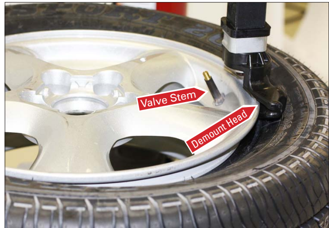
Figure 17 - Position Valve Stem Behind Demount Tool Tail
