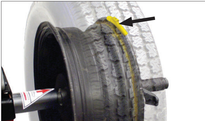
Figure 24 - Calibration Weight On Outboard Flange At Top-Dead-Center
