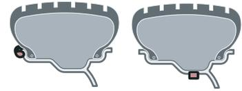
At the Clip 1 location, place the corrective weight amount at top-dead-center. If the T2 - Tape weight location is selected, the balancer activates its Laser Guided Operation™ feature (see page 6).
