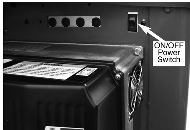
Figure 4 - On/Off Switch
