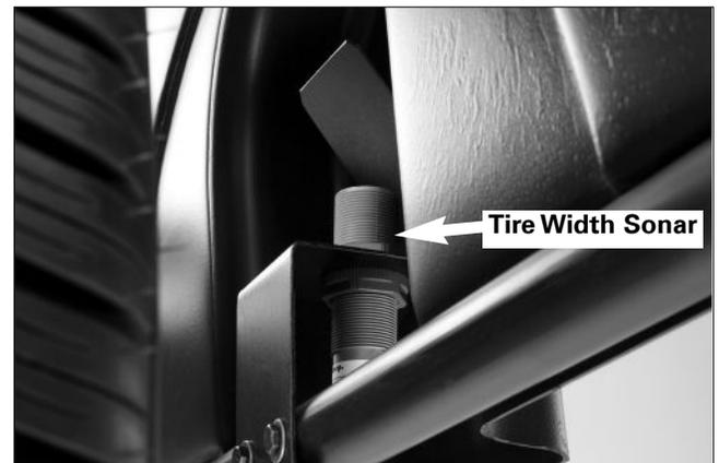
Figure 10 - Tire Width Sonar Located Inside Hood
