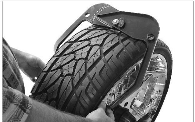
Figure 13 - Caliper Placement On Wheel
