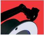
Place the round part of the gauge terminal on the flange as shown in the figure
