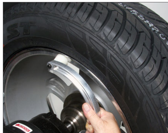
Figure 10 - Automatic A & D Measurement At Clip-on Weight Location
