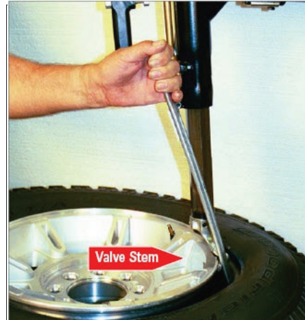
Figure 10 - Insert Bead Lifting Tool
