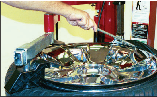
Figure 34 - Lift Bead Carefully onto Duckhead Tool
