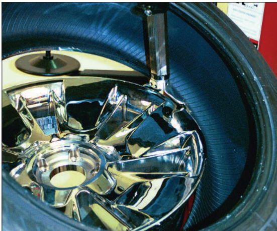
Figure 39 - Mount the Lower Bead
