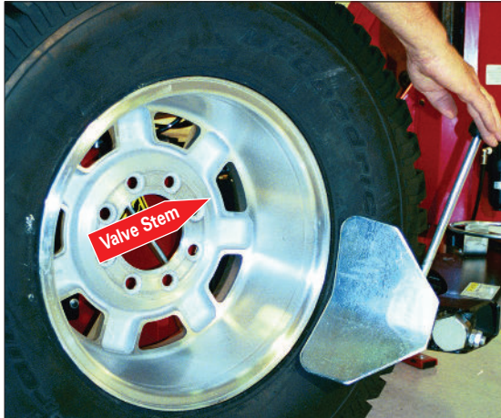
Figure 28 - Loosen Bottom Bead
