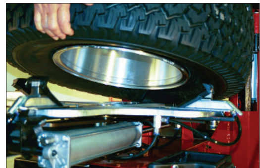
Figure 31B - Outside Clamped with Tire Removed
