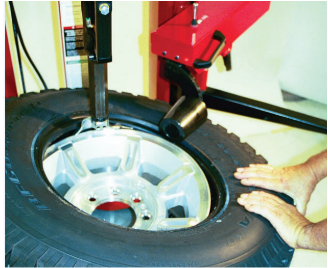
Figure 18 - Mounting Lower Bead
