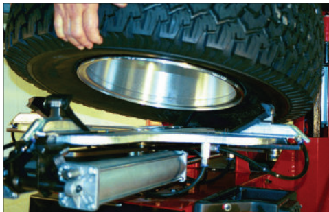
Figure 5 - Clamp Outside on Mag Wheels
