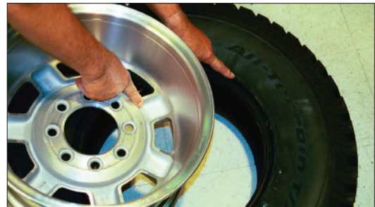
Figure 14 - Verify Size Match Between Tire and Wheel
