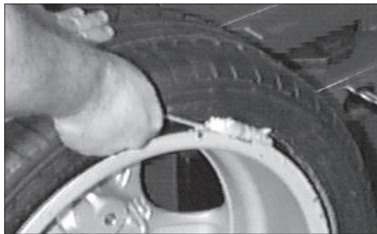
Figure 29 - Lubricate Bottom Bead
