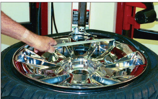
Figure 35 - Start Upper Bead Removal
