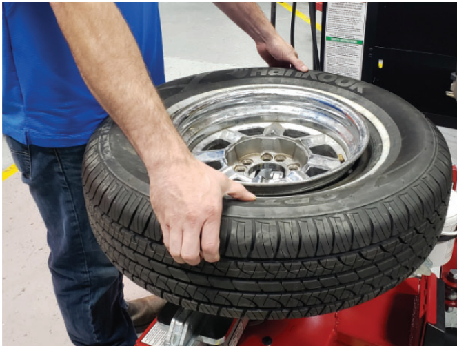
Figure 20 - Lift Tire Upwards for Bead Sealing
