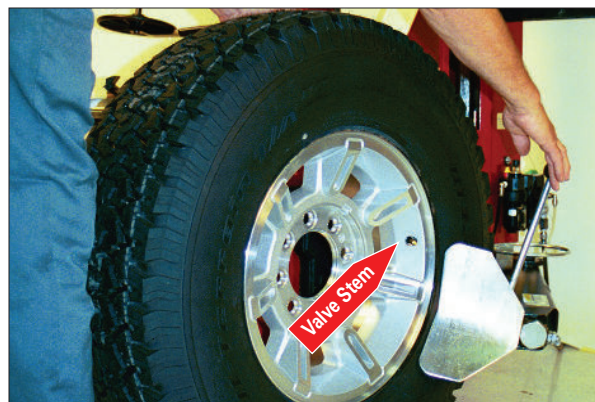
Figure 3 - Position Tire and Bead Loosener Shoe
