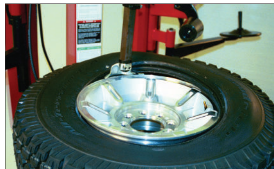
Figure 11 - Demount Upper Bead
