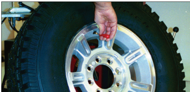
Figure 1 - Remove Valve Core to Deflate Tire
