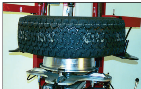
Figure 12 - Lift the Tire for Lower Bead Removal
