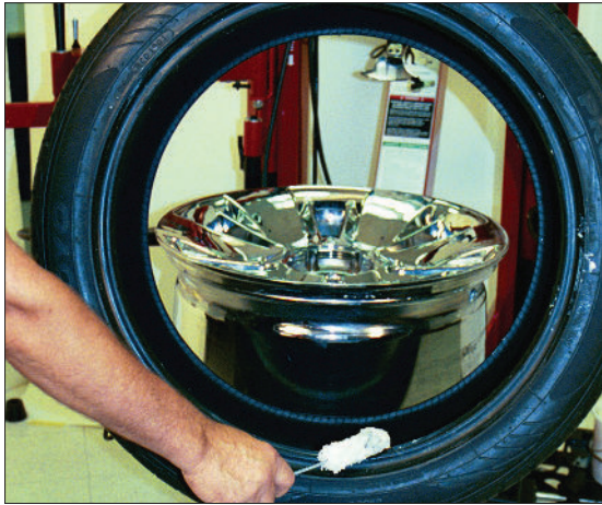
Figure 38 - Lubricate Tire Beads
