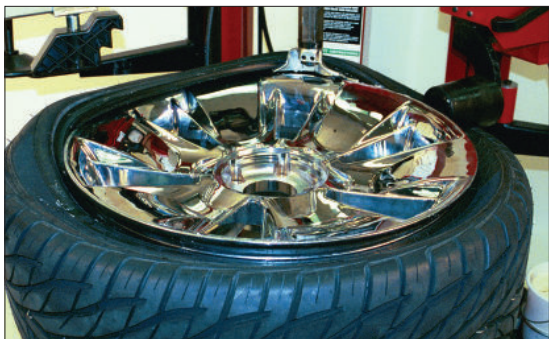
Figure 43 - The L.H. Helper Should Follow the Bead Lock
