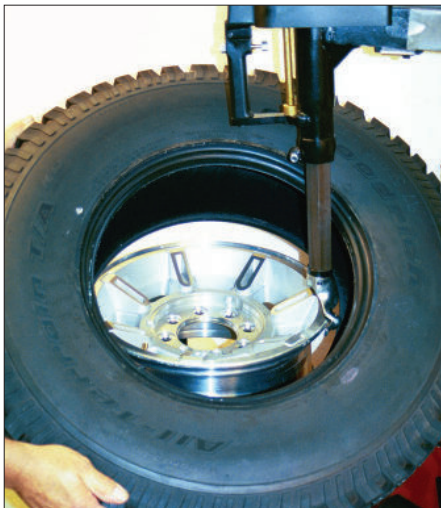
Figure 17 - Position Tire Against Duckhead Tool
