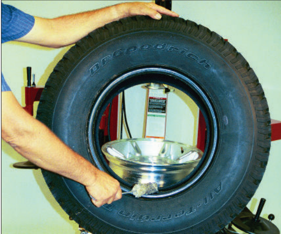
Figure 16 - Lubricate Tire Beads Liberally
