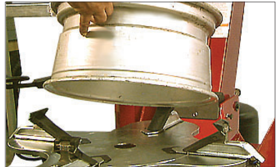
Figure 31A - Clamp Wheel (Tire Removed for Clarity)
