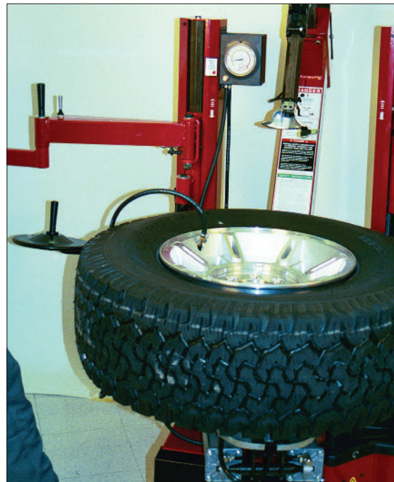
Figure 21 - Stand Back during Bead Seat
