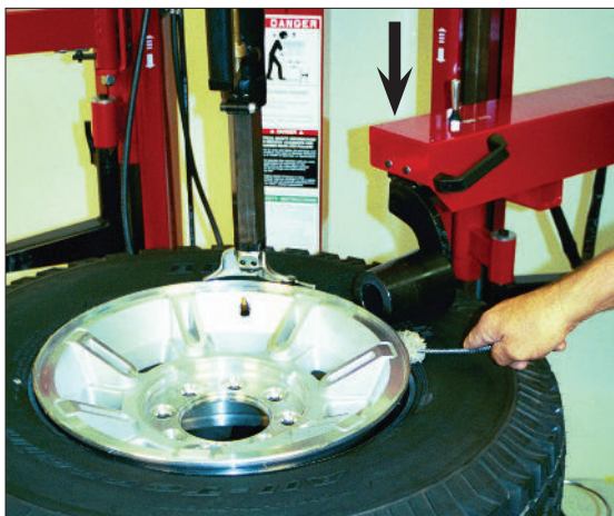
Figure 9 - Apply Rubber Lubricant to the Beads
