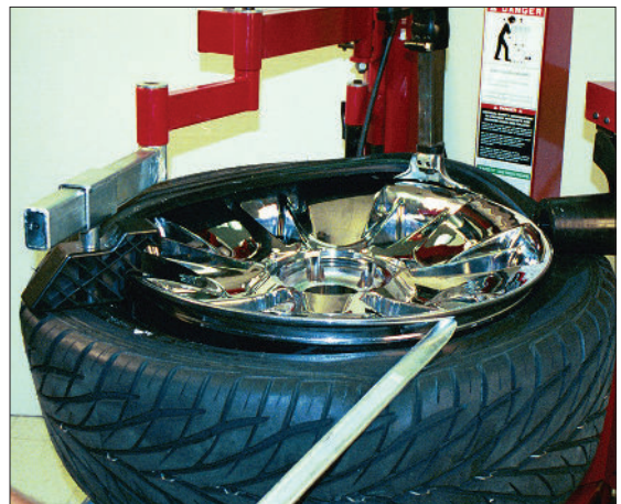
Figure 42 - Utilize the Lift Tool if Necessary
