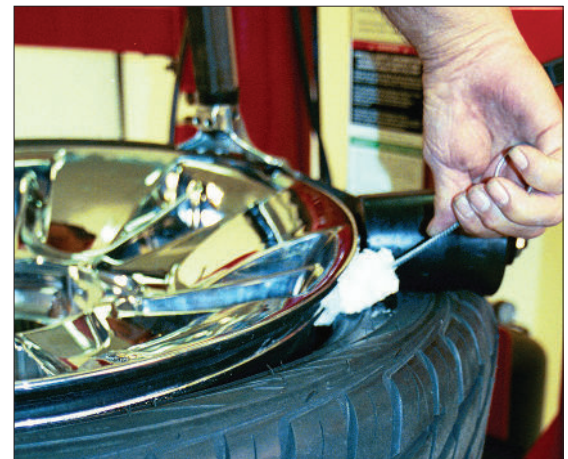
Figure 32 - Lubricate Upper Bead
