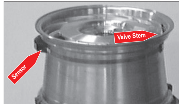
Figure 25 - Wheel with Strapped on Low Pressure Sensor/Transmitter
