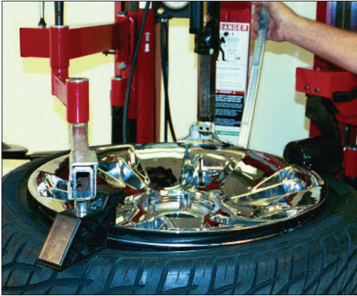
Figure 33 - Position Tire/Wheel for Demounting
