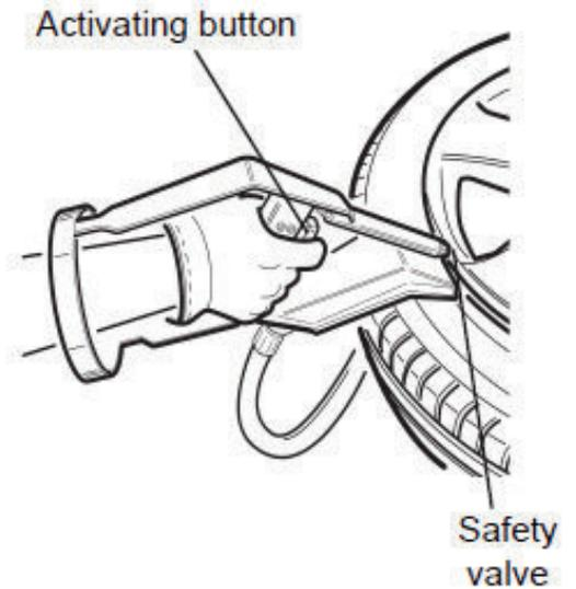
During the inflation stages (and especially during the bead seating operation), you must wear appropriate personal protective equipment to protect your hearing from possible blast injuries and from noise levels that sometimes exceed the permitted threshold.
