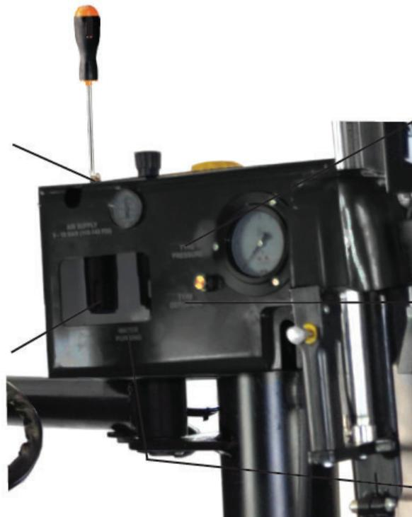
For long lasting correct functioning of the pressure limiter device, check on regular basis and discharge the condensation when needed.
