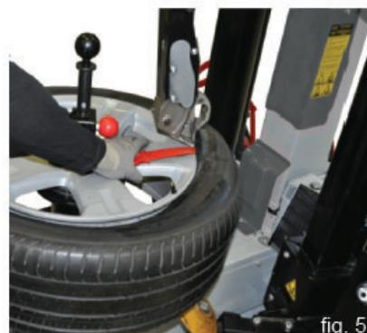
As soon as the bead is perfectly hooked, lift the mounting tool using the lever **20** to pull out the bead.
