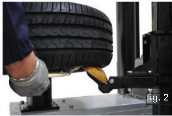
As soon as enough space is available, carefully apply tire lube paste to both to the rim inner surface and to the tire bead (fig. 2).
