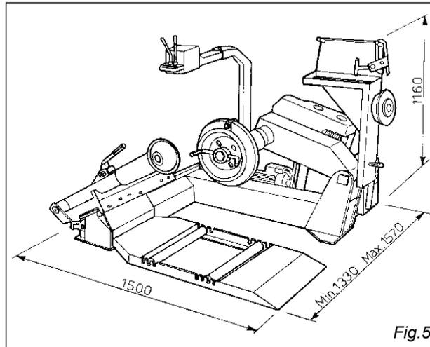
The tire-changer must be installed on a level concrete floor at least 6" (15 cm) thick, with a minimum concrete quality of B25 in compliance with DIN 1045 requirements (foundations). See the diagram herebelow.
