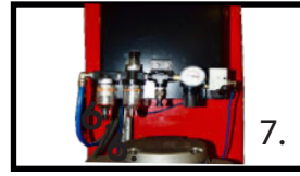
4. Air locking system with Filter/Regulator/ Lubricator standard
