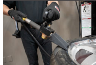
AUXILIARY BEAD SEALER (ABS) (PN 85606545)
