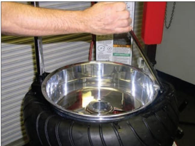
**110.** Once the bead is located on the duckhead, the lift tool maybe removed completely.
