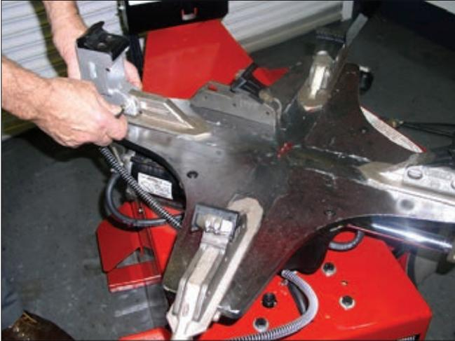
**103.** As with motorcycle clamps, after bead loosening and before clamping the wheel, preposition the clamps.
