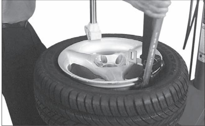
Figure 29 - Rotate Lifting Tool Down for Demount
