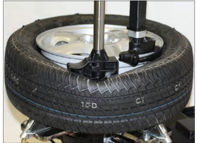
Figure 25 - Helper Foot Depressing Sidewall of Tire
