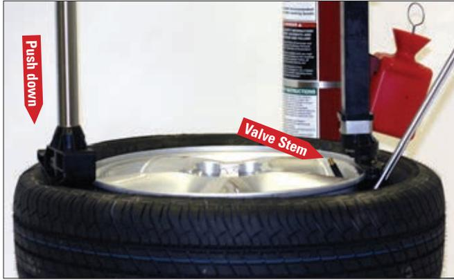
**108.** Before rotating the bead up and on the duckhead, use the Robo Arm to push the upper bead into the rim's drop center.
