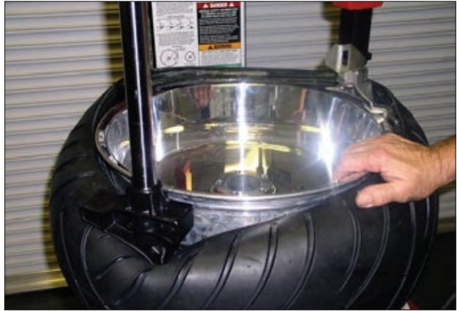
**206.** Reposition the RoboArm back to 90-degrees forward of the duckhead and finish the mounting.
