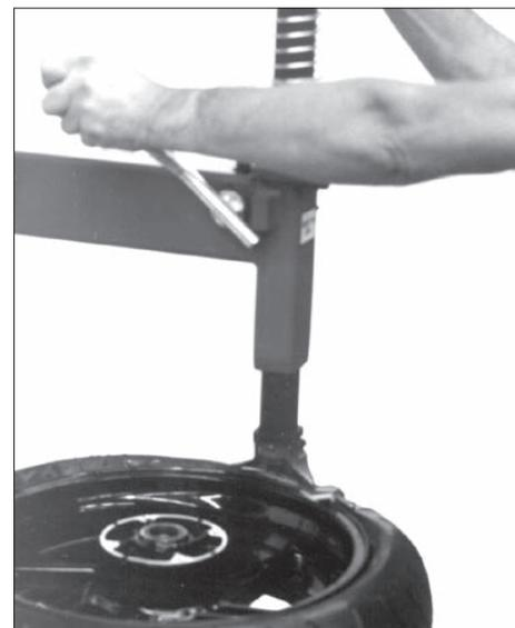
Figure 6 - Position Mount/Demount Tool
