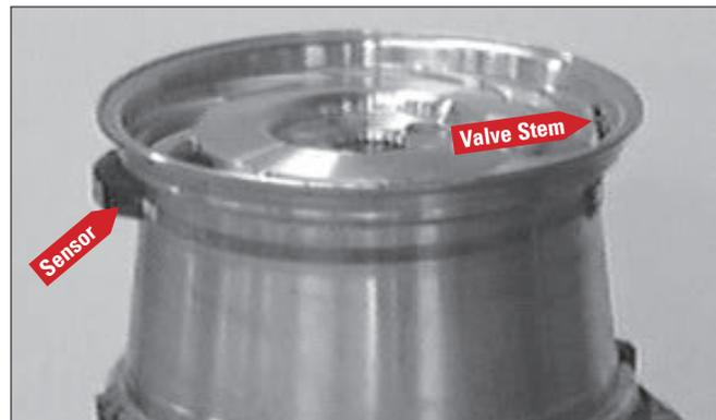
Figure 22 - Wheel with Low Pressure Sensor/Transmitter
