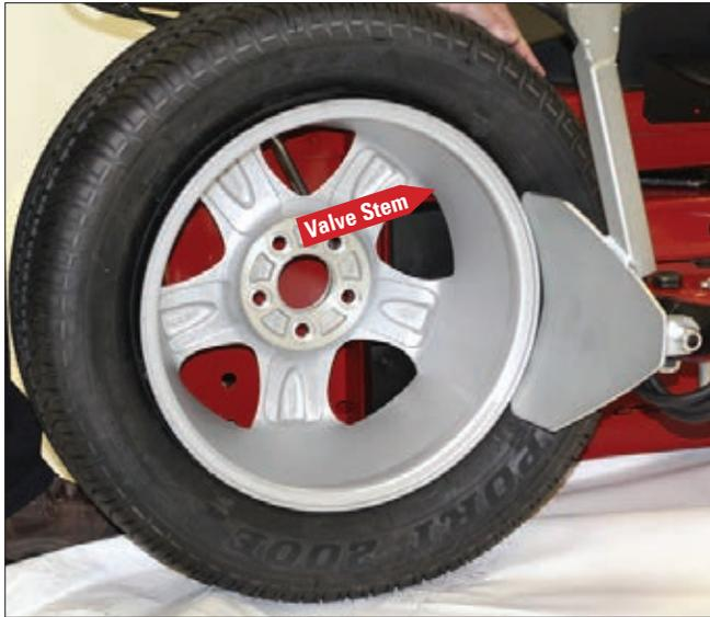
Figure 23 - Loosen Bottom Bead
