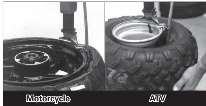
Figure 9 - Insert Bead Lifting Tool
