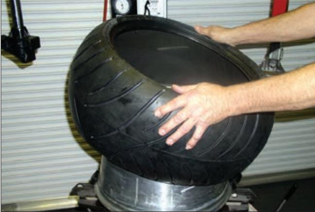
**202.** For the top bead, lubricate the bottom side of the top bead and the edge.
