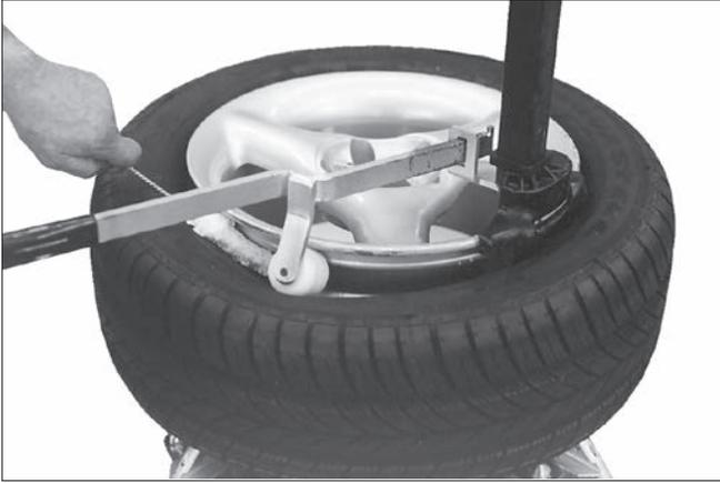
Figure 26 - Lubricate Upper Bead
