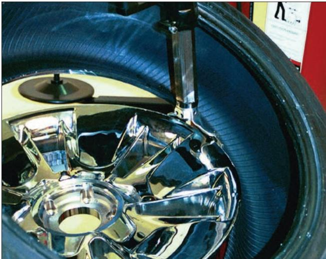
Figure 31 - Mount the Lower Bead
