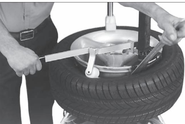
Figure 28 - Insert Bead Lifting Tool
