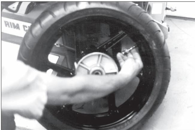
Figure 1 - Remove Valve Core to Deflate Tire
