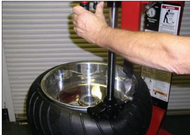
**106.** Lubricate the upper bead surface. To assist, position the manual roller assembly into the receiver. Press down and the roller between the rim and the tire bead. This will allow easy lubrication of the upper bead surface and rim flange.
