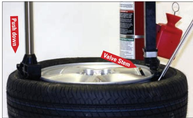
Figure 8a - Insert Bead Lifting Tool
