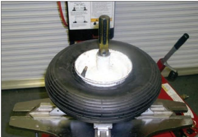
**B202.** Position the Snake™ tool and remove the top bead. Next remove the second bead.
