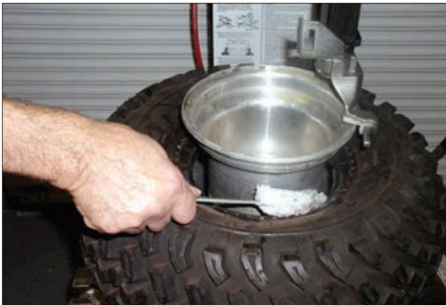
**A203.** Using typical procedures, remove upper bead.
