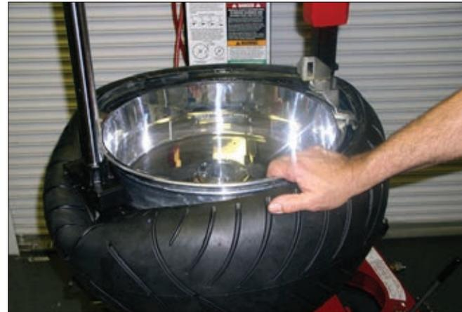
**207.** Use the RoboArm to push down on tire and swing duckhead from rim position.
