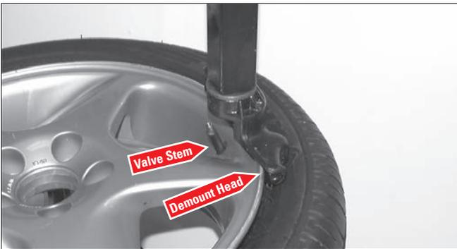
Figure 27 - Position Valve Stem Under Demount Head
