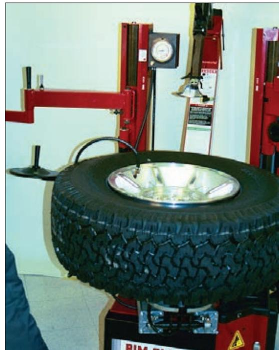
Figure 17 - Stand Back during Bead Seat
