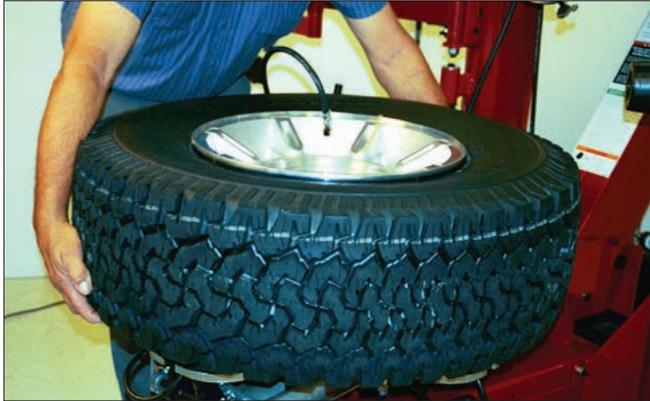
Figure 16 - Lift Tire Upwards for Bead Sealing
