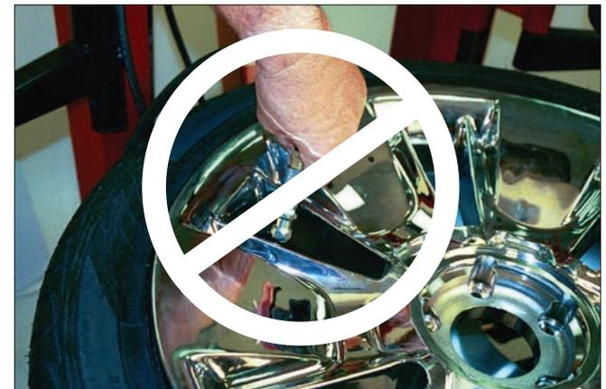
Figure 19 - Do Not Use a Hand-held Style Air Chuck
