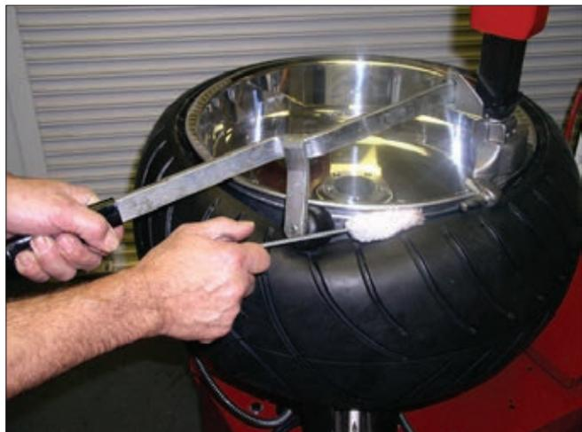
**107.** Insert the smooth curved end of the bead lifting tool over the forward end of the demount tool and below the top bead of the tire. Lift the bead up and over the knob on the demount tool. Also, note the valve stem position to the demount tool. Use the Robo-Arm® to push down on the tire opposite the demount tool to allow the bead to utilize the drop center area of the rim, this position reduces stresses in the bead and allows an easier bead lift.
