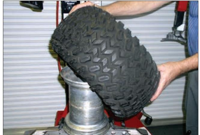
**A206.** Top bead is mounted using typical procedures.
