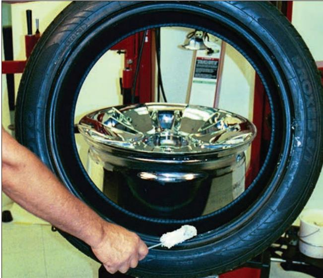
Figure 30 - Lubricate Tire Beads
