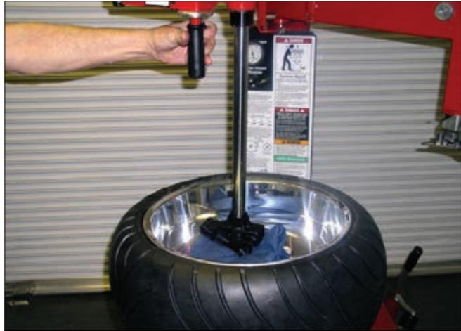
**105.** To assist in positioning the duckhead at the location near the rim, use the Robo Arm to press the tire sidewall down.
