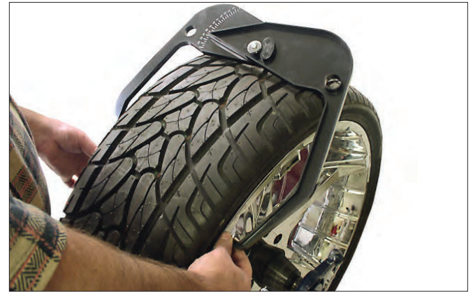
Figure 22 - Caliper Placement On Wheel
