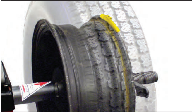
Figure 1 - Calibration Weight On Outside Flange At Top-Dead-Center
