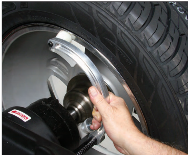
Figure 8A - Automatic A&D Measurement At Clip-on Weight Location
