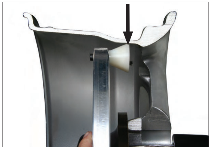
Figure 9A - Hidden Weight Location Viewed on a Cut Away Rim for Clarification.
