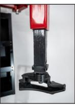
Tool used for mounting and demounting tires without damaging the rim.
