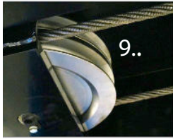
9. Unique cable routing uses a maximum of two pulleys stacked together with a trunion "non Rotation bar" that creates long cable & pulley life
