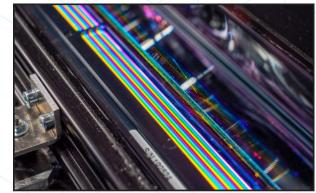
**Dedicated camera** Utilizing LEDs, the tread depth scanner picks up 300+ points to analyze tread depth.
